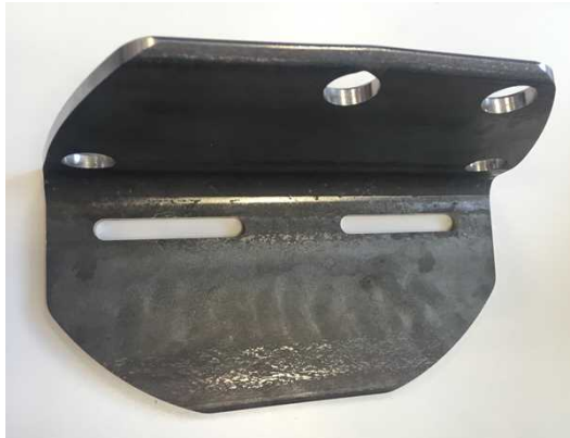
test sample without corrosion protection and deburring
